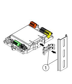
Series mounting using mounting feet supplied, on U-rail TS35
