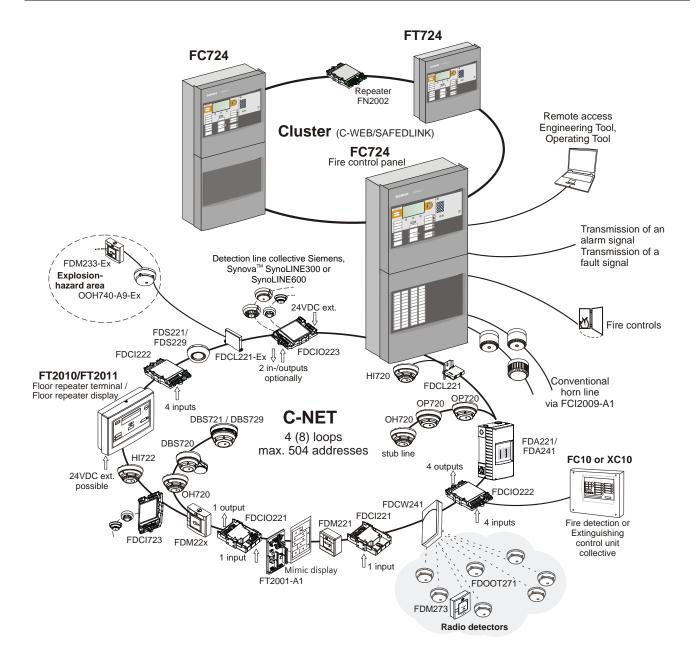
Up to 32 fire control panels und fire control terminals can be connected in a single cluster (C-WEB/SAFEDLINK) or up to 16 stations when the cluster is connected to a danger management system.
